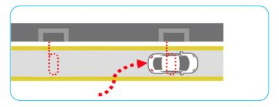
When a car enters in the middle of the lane, it is not detected by the first detection point, which prevents ZOOM Nitro Timer from tracking the total lane time for that car. By default, when a pull-in occurs, ZOOM Nitro Timer recognizes it and excludes the data for the car so that it does not skew calculated averages.
