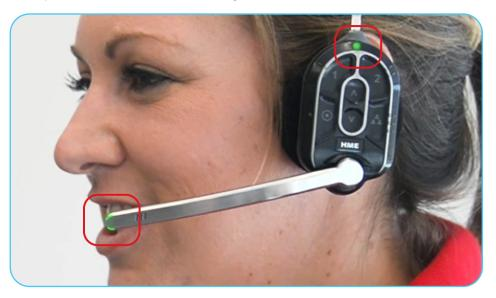
16. When communicating with Lane 2, the status LED above touch panel will **flash red**. The LEDs at the end of the microphone boom will illuminate **solid red**.
