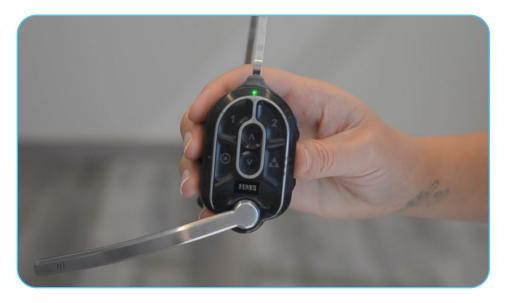
3. The headset is powered by a battery. Insert the battery in the area below the touch panel.
