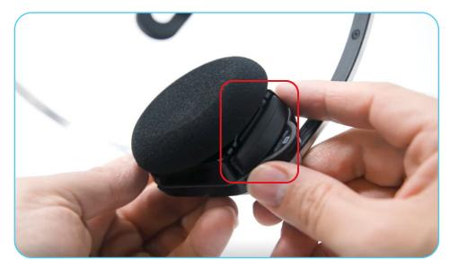
4. To remove the battery, press the **silver release button** above the earpad and pull down on the raised edge at the bottom of the battery.
