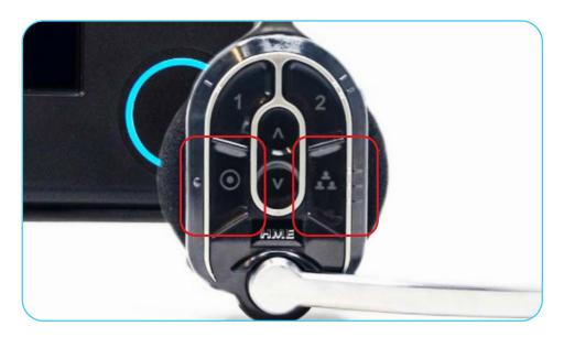
12. The **Master Volume Control** is located in the center. Tap the **Up** or **Down arrows** to increase or decrease the headset volume. **Note**: You will hear a **'beep'** as you adjust the volume. The volume and pitch of the beep will decrease or increase with each adjustment.
