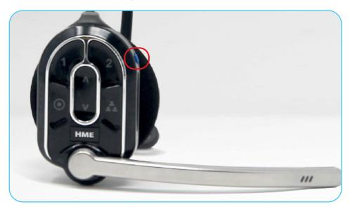
2. When the headset has been paired to the Base Station, ensure you hold the headset by the outer edge to avoid unintentionally tapping the interface.
