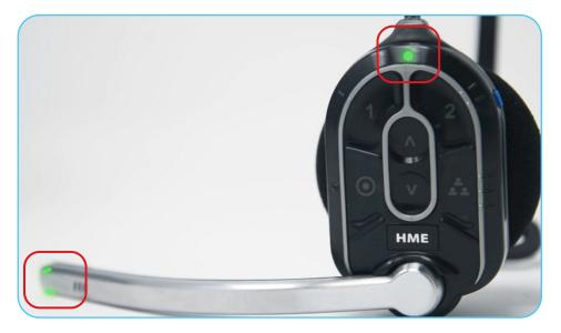
15. When communicating with Lane 1, the status LED above the touch panel will **flash green**. The LEDs at the end of the microphone boom will illuminate **solid green**.
