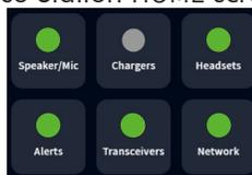
**Note:** The AC70 requires close physical proximity (<10 ft (3 m)) to the base station if you desire to monitor battery status via the base station HOME screen. When within range, the **Chargers** indicator on the HOME screen changes from to (gray to green). Once green, tap **Chargers** to view battery status.
