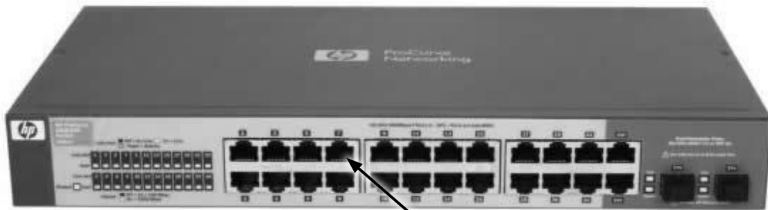
Figure 8: 24 Port Network Switch
