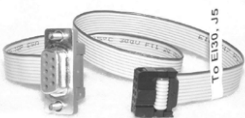
Flat-ribbon serial cable
