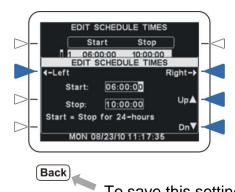
4. Select the (-Left and Right-) arrows to highlight a number in the Start or Stop field that you want to change. As the highlight passes the end of either field, it will move into the other. Select the Up ▲ and Dn ▼ arrows for higher or lower numbers.
