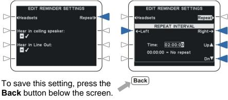
2. To set the time interval between repeats, select the (-Left and Right-) arrows to highlight the numeral in the Time field that you want to change (HH:MM:SS, where HH = hours, MM = minutes and SS = seconds). Select the Up ▲ and Dn ▼ arrows for higher or lower numbers. If you do not want the message to repeat, set all zeros in the Time field.
