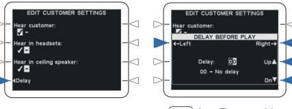
2. To set the number of seconds delay, select the **(-Left** and **Right-)** arrows to highlight the number in the Delay field that you want to change. Select the Up ▲ and Dn ▼ arrows for higher or lower numbers.
