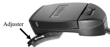
Figure 6. Headset size adjustment
