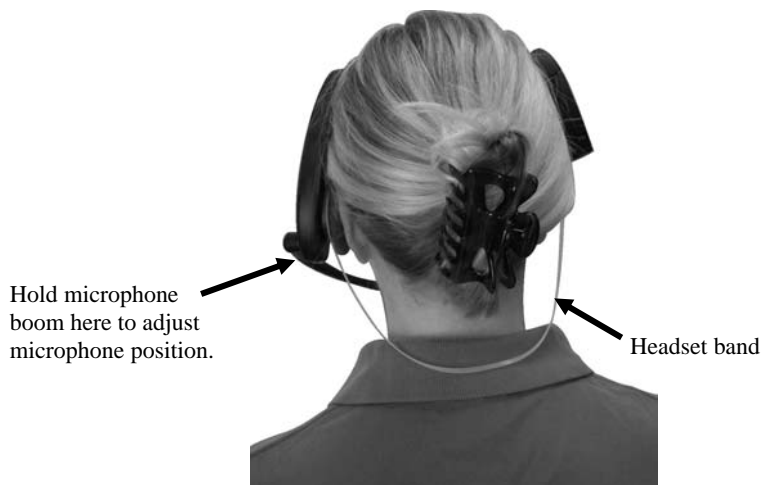
Figure 7. Correct wearing of the headset
