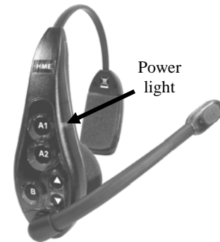
Figure 2. Headset buttons and power light
