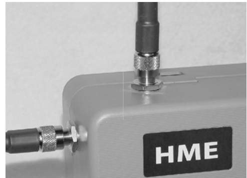
Figure 1. Antenna cable connectors
