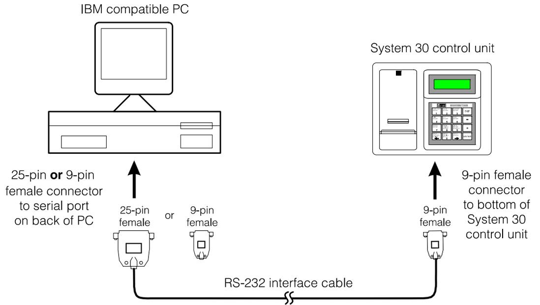
**Figure 4. PC to System 30 Timer direct serial cable connections**
