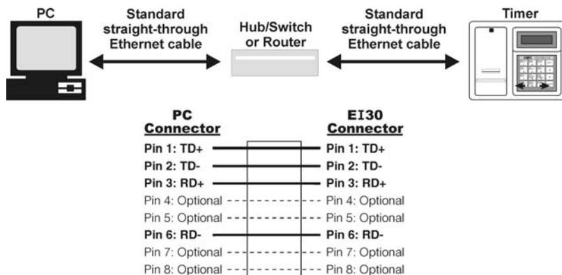
Figure 2. Computer connected via hub/switch or router to a network-enabled System 30 Timer (EI30)
