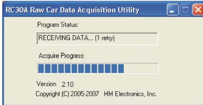
While the RC30A™ is collecting data, this screen will show activity in the Acquire Progress bar. As data is received from the Timer, the Program Status bar will show the number of Raw Car Data records received.
