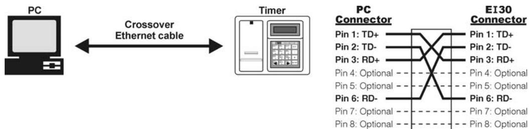
Figure 1. Computer connected directly to a network-enabled System 30 Timer (EI30)
