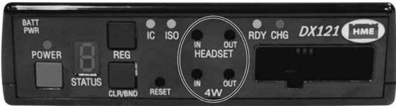
Base Station front panel showing HEADSET and 4W (4-Wire) input and output level adjustments
