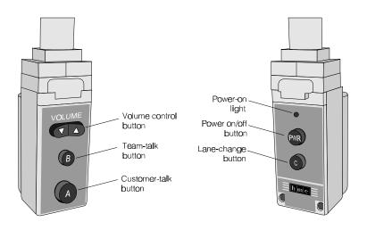
Figure 3. COM400CC control buttons.
