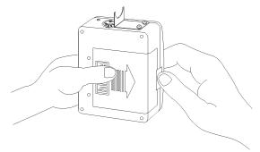
Figure 17. Opening the battery compartment
