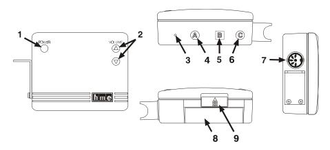
Figure 12. COM400BP controls, connector and indicator light
