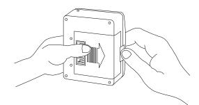
Figure 25. Opening the COM430BP battery compartment
