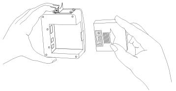
Figure 16. Installing the battery
