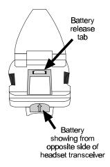
Figure 27. HS30 Headset transceiver
