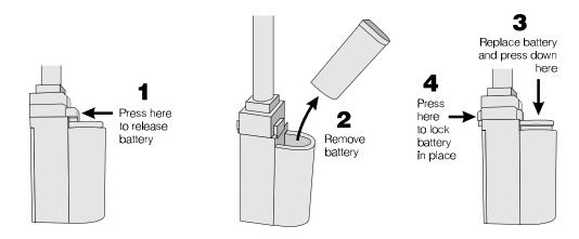
Figure 6. Remove and replace Communicator battery
