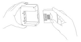
Figure 24. Installing the COM430BP battery
