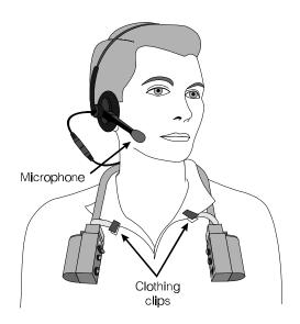
Figure 5. Correct wearing of the COM400CC
