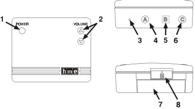
Figure 21. Communicator controls
